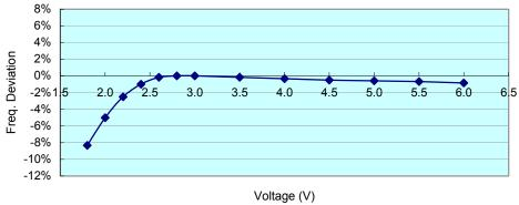
Voltage vs Freq. Deviation (6.0KHz@3V)
